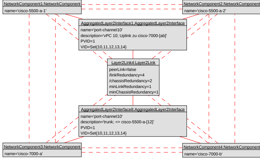
Fig. 4. Object diagram of four interconnected network switches in the University of Bremen data center with hidden layer 1 objects. With the derived properties, all necessary information is visible.
